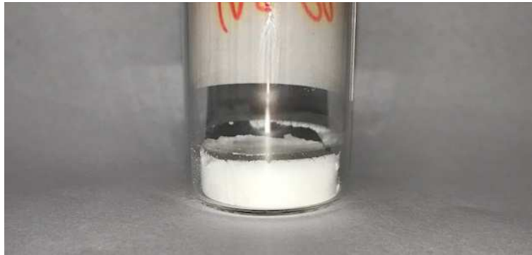
FIG. 2: Lactose cake with visible shrinkage effect
