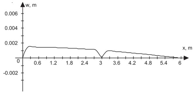
Fig. 15. Distribution of the cylindrical wall deflection over the tank length for 23rd coupled mode.
