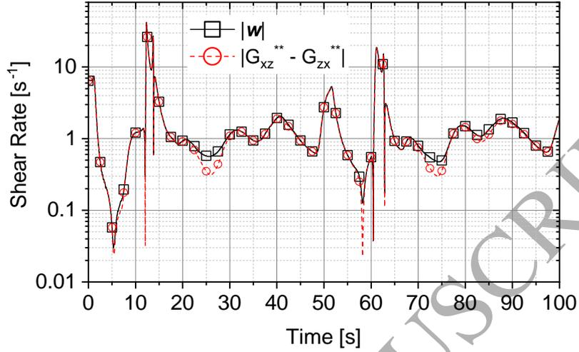
Figure 17: Time evolution of the shear rates at the coordinate system  $e_i^{**}$  and the magnitude of vorticity along the particle trajectory; the spherical particle is tracked by including the action of the lift force on the particle calculated by the present model (tracking time: 100 s, time step:  $10 \mu s$ ,  $D_p = 100 \mu m$ ).
