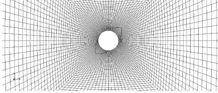
Figure 5: The mesh around a fully-resolved free-rotating spherical particle.
