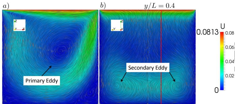
Figure 8: Numerically computed flow streamlines of a 3D lid-driven cavity flow in a cube; a) the longitudinal plane  $y/L = 0.4$ ; b) the central transverse plane  $x/L = 0.5$ ; the red line indicates the plane of particle tracking  $y/L = 0.4$ ;  $U$  is the magnitude of the fluid velocity ( $Re = 470$ , the dimension of the domain:  $L = 0.1 m$ ) (Cui et al., 2018b).
