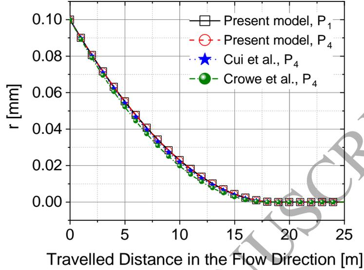
Figure 3: Translational motion of a spherical particle in Poiseuille flow for different shear lift force models and initial positions (tracking time: 50 s, time step: 10  $\mu$ s,  $D_p = 20 \mu$ m).
