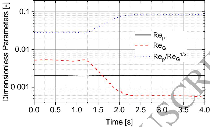
Figure 10: Time evolution of dimensionless parameters of a spherical particle moving in the lid-driven cavity flow (tracking time: 4 s, time step:  $10 \mu s$ ,  $D_p = 100 \mu m$ ).
